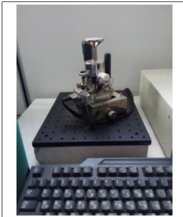
Figure 8. Atomic Force Microscope (Topometrix, Santa Clara, USA), available in the Micro/NanoTechnology Center , equipped with a specially modified optical probe operated in non-contact and contact modes for 3D Measurement and 2D Measurement.
