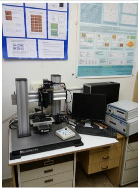
Figure 3. 3D Micro Measurement System available at the Micro/NanoTechnology Center for 3D and 2D Characterization.
